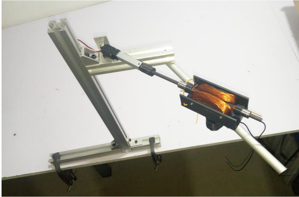
Fig. 7. Photograph of the experimental one Degree of Freedom arm to characterize the MR linear clutch
