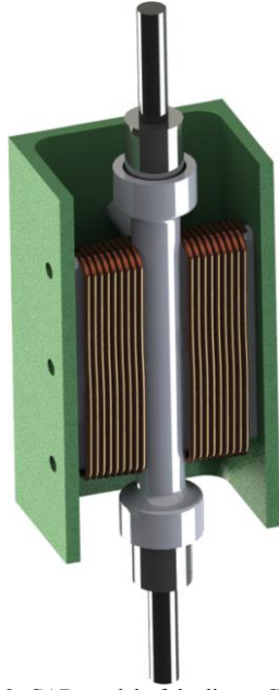
Fig. 2. CAD model of the linear Clutch
